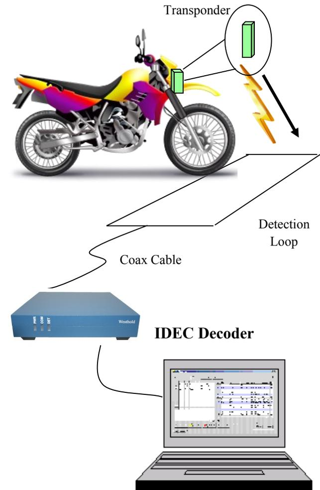
1. When transponder goes over activation loop, it is detected by IDEC decoder
