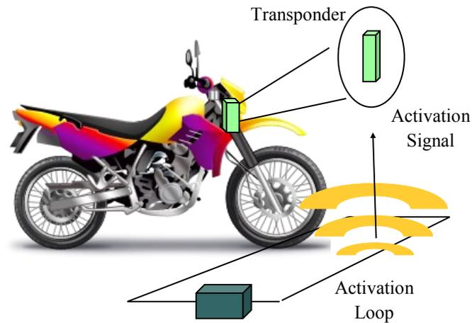
1. Activation signal turns transponder on.
